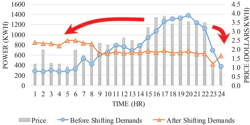
Figure 2.1: Shifting the non-urgent power demands from peak time to off-peak time
