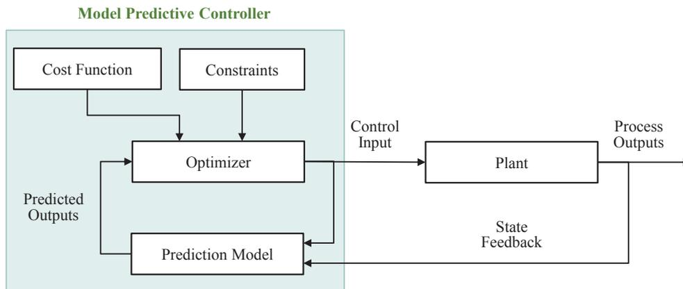
Figure 2.4: State feedback for Model Predictive Controller
