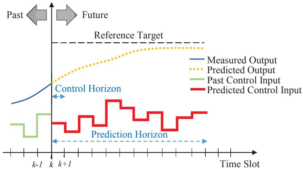
Figure 2.3: Basic concept for Model Predictive Control
