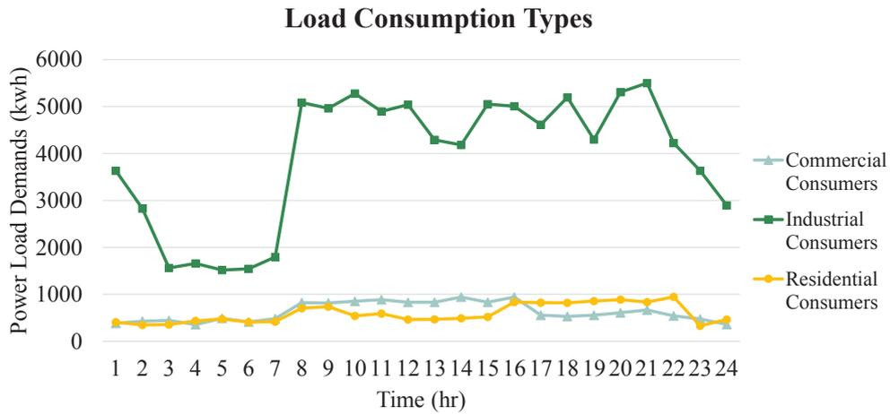
Figure 5.1: Type of power consumers in a smart grids
