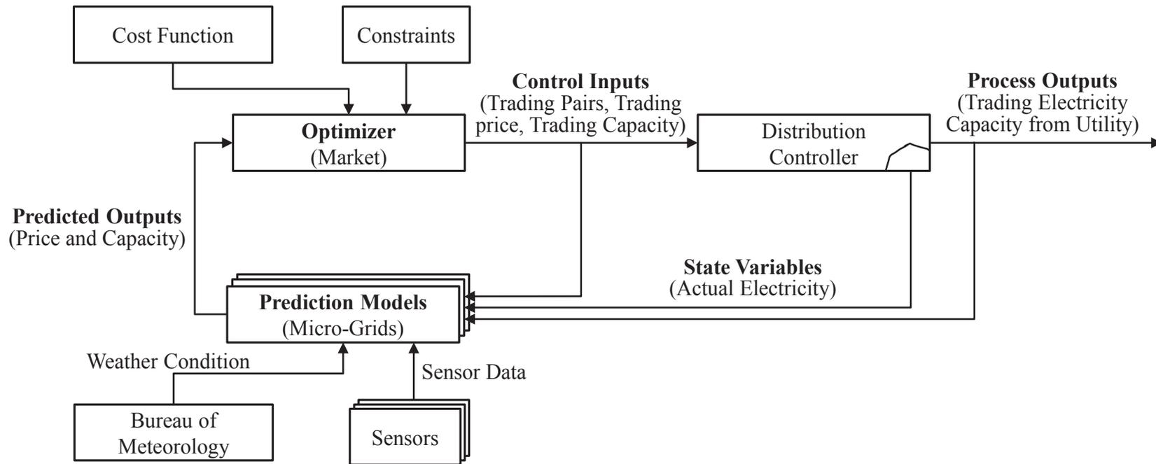
Figure 4.1: Architecture of Model Predictive Control based Distribution Management System
