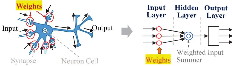
Figure 2.5: A model of an artificial neuron
