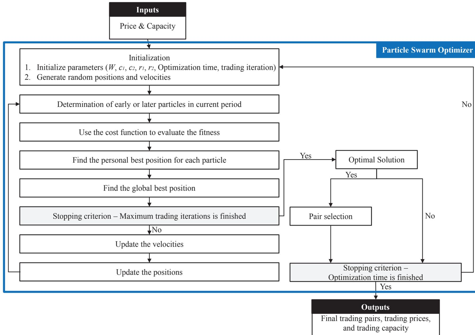
Figure 4.8: The Particle Swarm Optimizer
